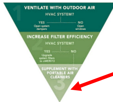
Figure 2. Illustration of the order in which to consider improvements to ventilation in buildings. 2
